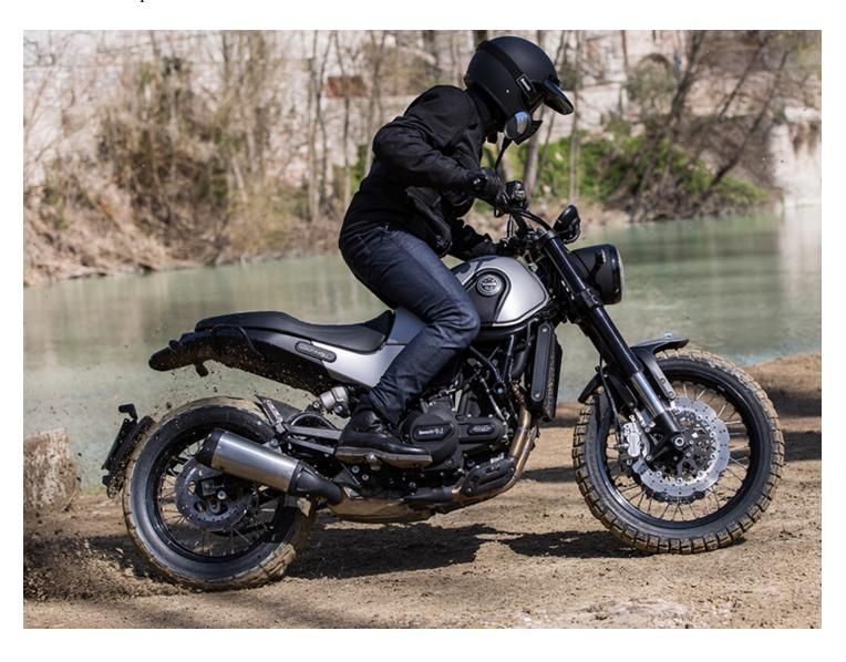
Leoncino Trail is the "all-terrain" version of the House of Pesaro's twin-cylinder, a dynamic and sporty motorcycle designed for pure fun in all riding conditions. This Benelli model shares the engine of the street bike, a 500 cc four-stroke twin-cylinder that is liquid-cooled, with a power output of 47,6 hp (35 kW) at 8500 rpm and torque of 46 Nm (4.6 kgm) at 6000 rpm. <br/>
